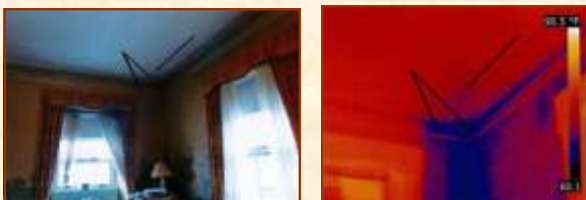
Executive Director's Office Large cooler area where two external walls meet, small dark circular area
